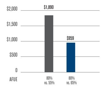
Three-Year Heating Savings of compared units - dollar amounts computed at \$.092 ccf, for 2,500 full-load heating hours and a system rated at 60,000 Btuh. Actual savings vary depending on climate conditions, fuel rates, and patterns of usage according to individual lifestyle.
